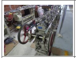
NC Photo No-01 Belt cover was missing with auto placket machines
